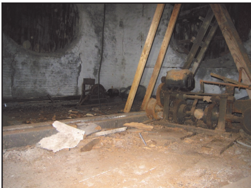
4th Level before bell tower, machinery used to ring original bell on lawn
